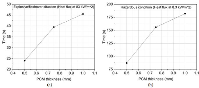
**Figure 4.** Effects of PCM thickness variations on glove thermal protection performance (times to second-degree skin burn temperature (60°C)) for (a) explosive/flashover situation (heat flux at 83 kW/m<sup>2</sup>) and (b) hazardous condition (heat flux at 8.3 kW/m<sup>2</sup>) (PCM at location L3).
