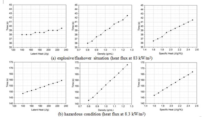
**Figure 3.** Times to second-degree skin burn temperature (60°C) - Effects of latent heat, density, and specific heat variations on glove thermal insulation performances for (a) explosive/flashover situation (heat flux at 83 kW/m<sup>2</sup>) and (b) hazardous condition (heat flux at 8.3 kW/m<sup>2</sup>).
