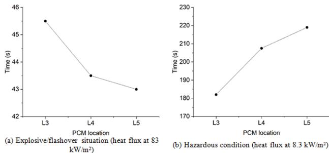
**Figure 5.** Effects of PCM layer location variations on glove thermal protection performance (times to second-degree skin burn temperature (60°C)) for (a) explosive/flashover situation (heat flux at 83 kW/m<sup>2</sup>) and (b) hazardous condition (heat flux at 8.3 kW/m<sup>2</sup>) (PCM thickness of 1 mm).
