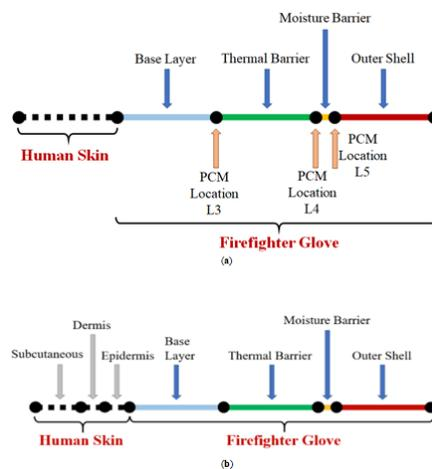
**Figure 1.** 1D numerical modeling geometry for a typical structural firefighter glove: (a) considering average skin thickness (no bioheat transfer) – no blood circulation; (b) considering bioheat transfer in human skin (epidermis, dermis, and subcutaneous layers) – considering blood circulation.
