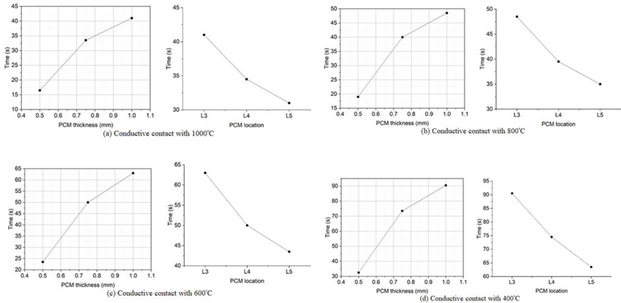
**Figure 6.** Effects of PCM layer thickness and location variations on glove thermal protection performance (times to second-degree skin burn temperature (60°C)) under (a) conductive contact at 1000°C, (b) conductive contact at 800°C, (c) conductive contact at 600°C, and (d) conductive contact at 400°C. (For the studies on PCM thickness effect, the PCM layer location was set at L3; for the studies on PCM location effect, the PCM thickness was set at 1 mm.)
