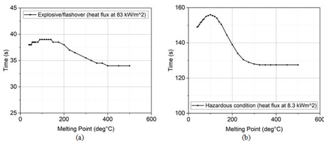
**Figure 2.** Time to second-degree skin burn temperature (60°C) under different  $T_m$  of PCM for (a) explosive/flashover situation (heat flux at 83 kW/m<sup>2</sup>) and (b) hazardous condition (heat flux at 8.3 kW/m<sup>2</sup>).
