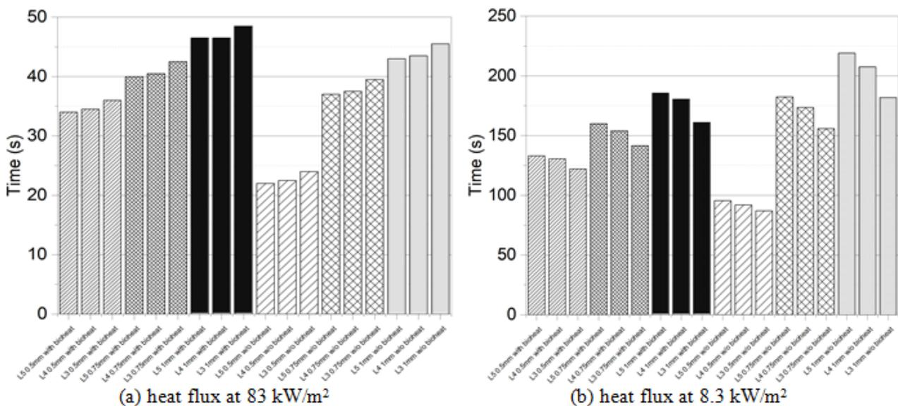
**Figure 7.** Times to second-degree skin burn temperature (60°C), considering the effect of skin bioheat transfer (blood circulation), under (a) explosive/flashover situation (heat flux at 83 kW/m<sup>2</sup>) and (b) hazardous condition (heat flux at 8.3 kW/m<sup>2</sup>). The x-axis shows the location and thickness of PCM layer in firefighters' glove.
